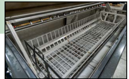
Interior Basket Assembly with Oscillating Spray Manifold
