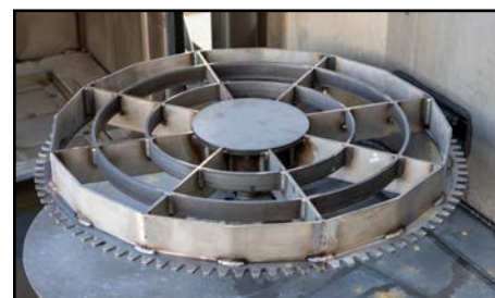
Heavy Duty Gear-Driven Turntable Assembly
